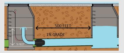
**Stay out of the Danger Zone:** Either with water or air, never inflate or deflate a pipe plug unless you are outside of the Danger Zone.
